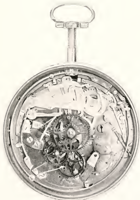
No. 6. Watch No. 148. WORKS UNDER DIAL. "PERPETUELLE" WATCH.
